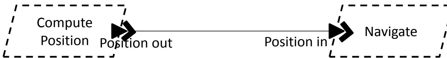
➤ Properties are used to tune the behavior of the event-data port (queue\_size, overriding, etc.)
